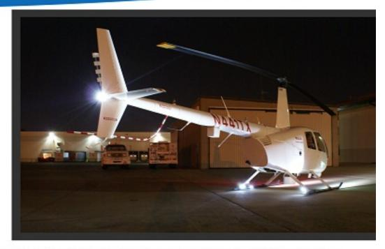
Beneficial in a variety of situations, from the heliport to darkened landing zones to the air, DeVore Aviation lighting systems provide a tangible advantage to the visibility of your helicopter and the safety of your operations. TEL-TAIL lighting fixtures enhance airborne identification by illuminating the entirety of the aircraft, enabling instant recognition in high traffic situations.
